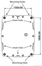
The mounting plate in the application must cover the entire top plate of the BL1 and be strong enough to carry the load.
