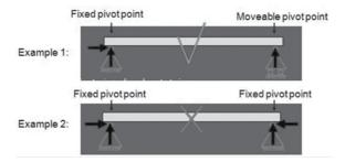
The reason why it is important only to fix one column is that the columns will not move exactly in parallel – even if you have positioning such as hall.
