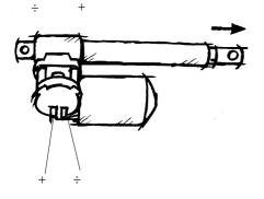
LA30 Actuator with reed ( only possible with 24V L-motor )
