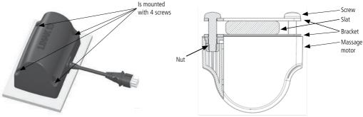
Mounting of the screw with max. torque 2 Nm
